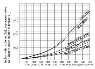
Standard cubic feet per hour. Cubic meters per hour in brackets  $[\ ].$
