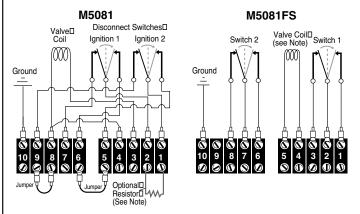
**NOTE:** For grounding the ignition (CD models only) through the fuel valve's internal snap-switch, a Murphy Magnetic Switch adapter (see page 4) must be used in addition to a 100 ohm, 2 watt resistor (supplied with valve).
